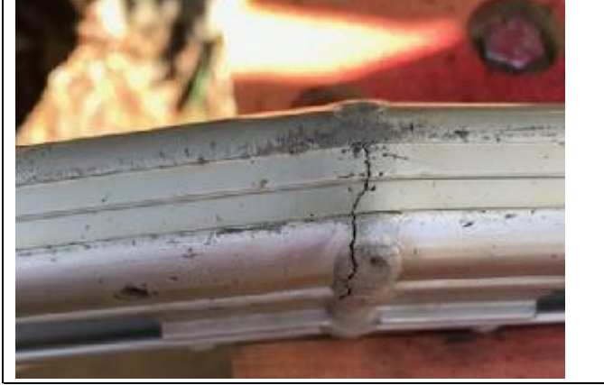
Crack in Tiller Arm (get it welded (again))
